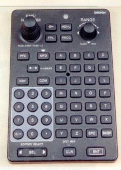
With its Jumbotron-like MFD and crisp, synthentic-vison PFDs, the Garmin G1000 transforms the Meridian. The GFC 700 autopilot is especially well suited to the airplane. The new console-mounted keypad (above) eases pilot workload by simplifying data input to the com radios and the nav system.
